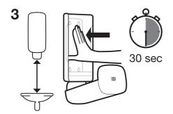
Mount the dispenser to the flat surface, press firmly and hold in place for at least 30 seconds.
